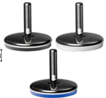
**Base material:** Internal part made of reinforced polyamide; external covering made of stainless steel AISI 304; anti-slip pad made of thermoplastic rubber 68 Shore black, white or blue Ral 5005 colour.
